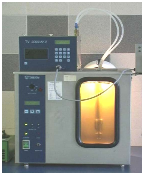
Obr. 1 Poloautomatický viskozimeter TAMSON TV 200/AKV na stanovenie kinematickej viskozity Fig. 1 Semi-automatic viscometer TAMSON TV 200/AKV for determination kinematical viscosity
